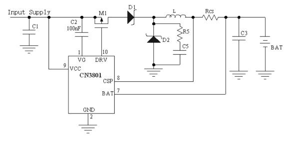
Figure 4 high frequency oscillation suppression
