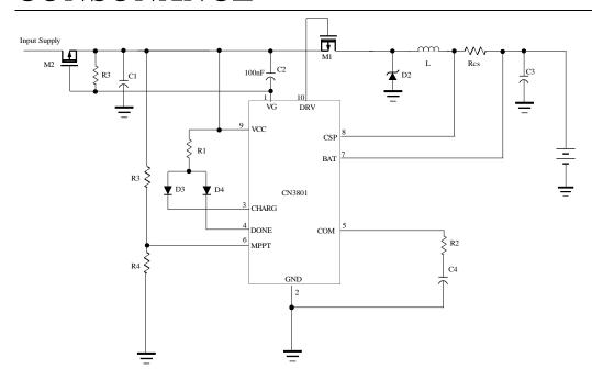
Figure 3 using PMOS to realize power reverse connection protection and
