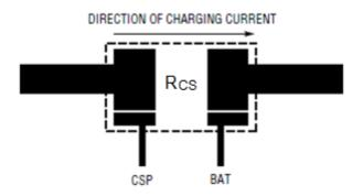
Figure 5 Kelvin Sensing of Charge Current
