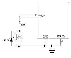
Figure 3 Using Battery Temperature Monitoring Function
