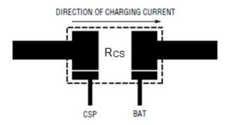
Figure 5 Kelvin Sensing of Charge Current
