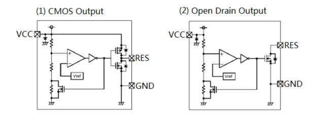
Figure 2 Block Diagram
