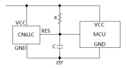
Figure 4 Power-on Reset Circuit
